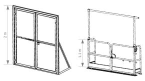
Landing gates with interlocking device
